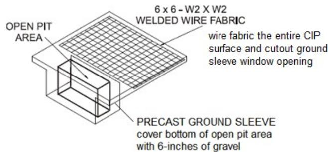
Transformer pad will be 9 inches thick minimum with welded wire fabric and #4 reinforcing bars. See site specific pad dimensions furnished by Clemson University Utilities for each transformer location.
