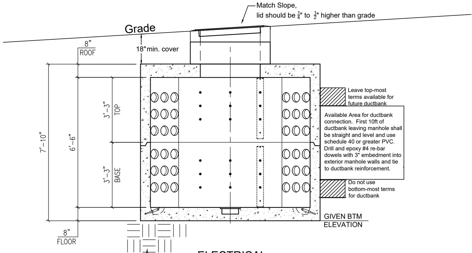
CONTRACTOR SHALL SET MANHOLES ON A LEVEL AND COMPACT BEARING SURFACE
